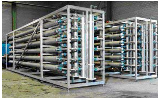
Ultra filtration for drinking water treatment
